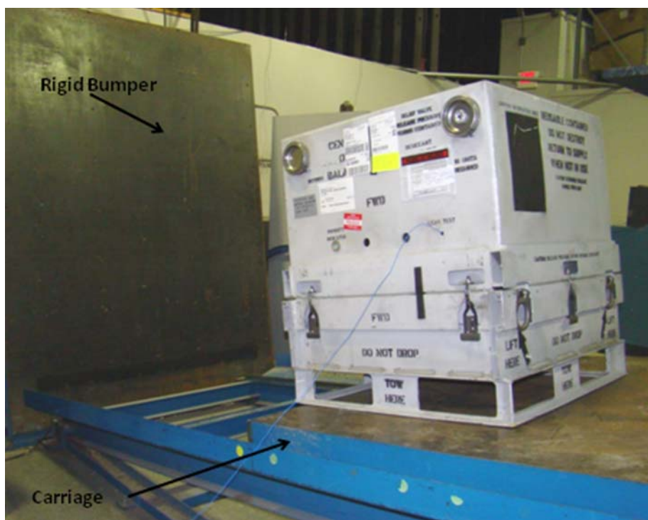
FIGURE 20. Incline impact test setup.
